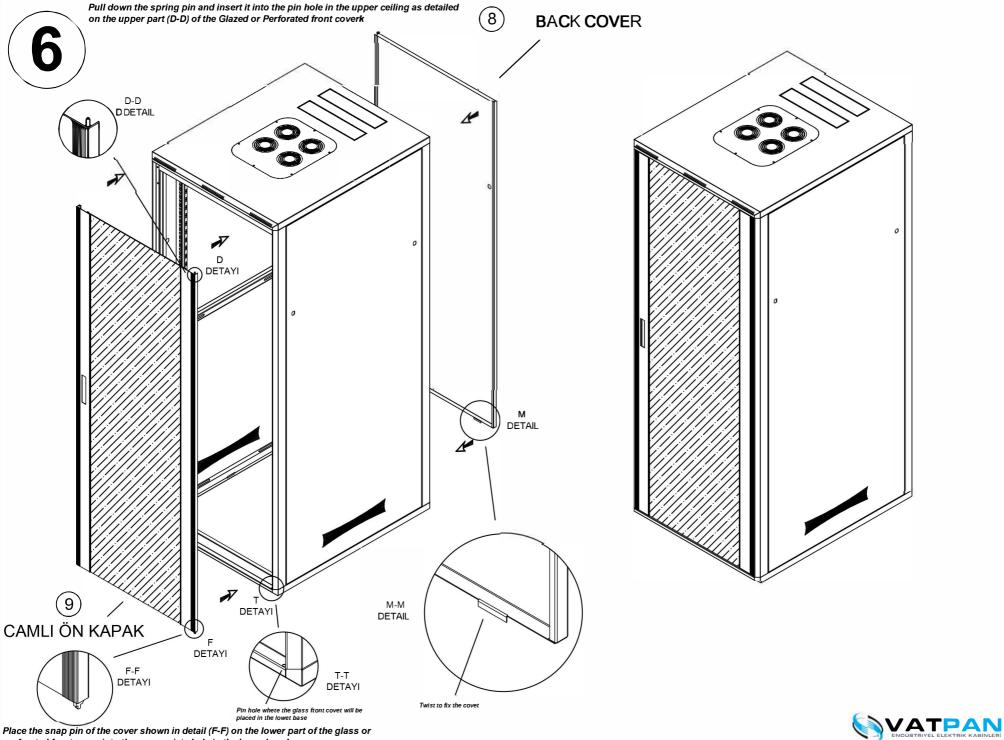
Place the snap pin of the cover shown in detail (F-F) on the lower part of the glass or perforated front cover into the appropriate hole in the lower basek
